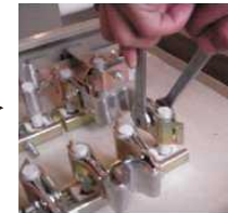
(2) 拧下需更换的硅钼棒夹头螺丝
